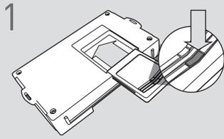
1 Slide cartridge into unit. Notice button under LED.
