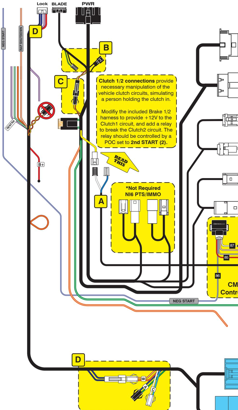
**Clutch 1/2 connections** provide necessary manipulation of the vehicle clutch circuits, simulating a person holding the clutch in.
