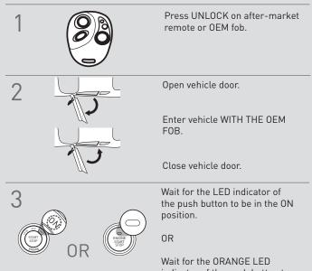
Wait for the ORANGE LED indicator of the push button to turn on.
