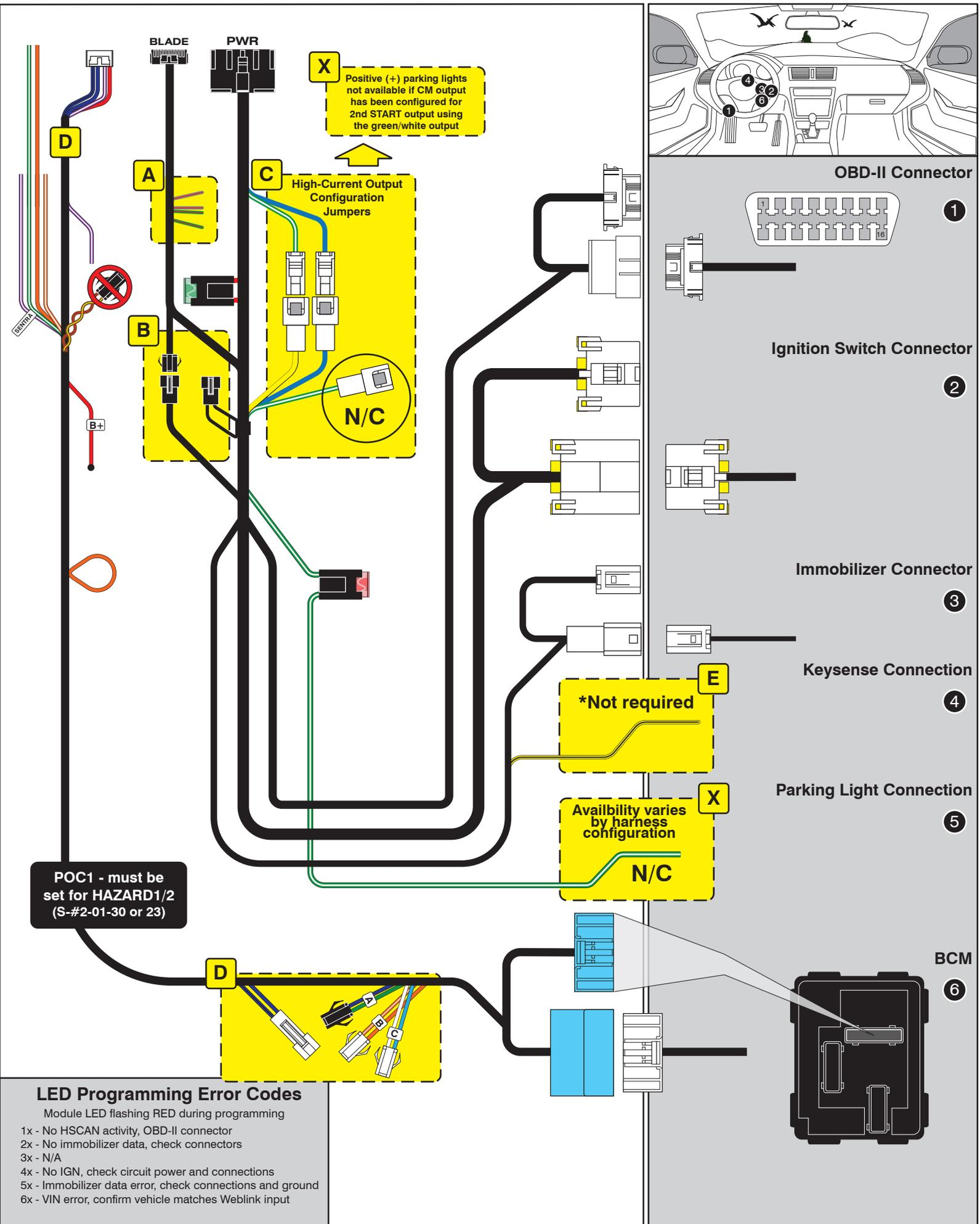
**X** Positive (+) parking lights not available if CM output has been configured for 2nd START output using the green/white output
