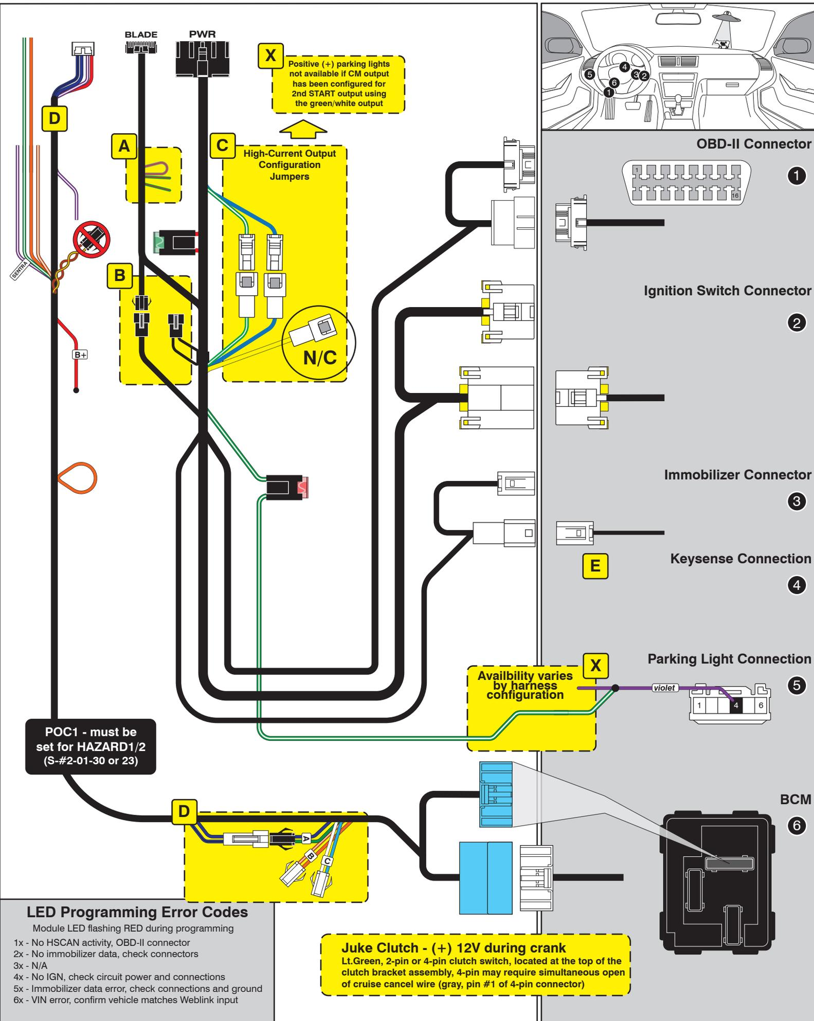
**X** Positive (+) parking lights not available if CM output has been configured for 2nd START output using the green/white output
