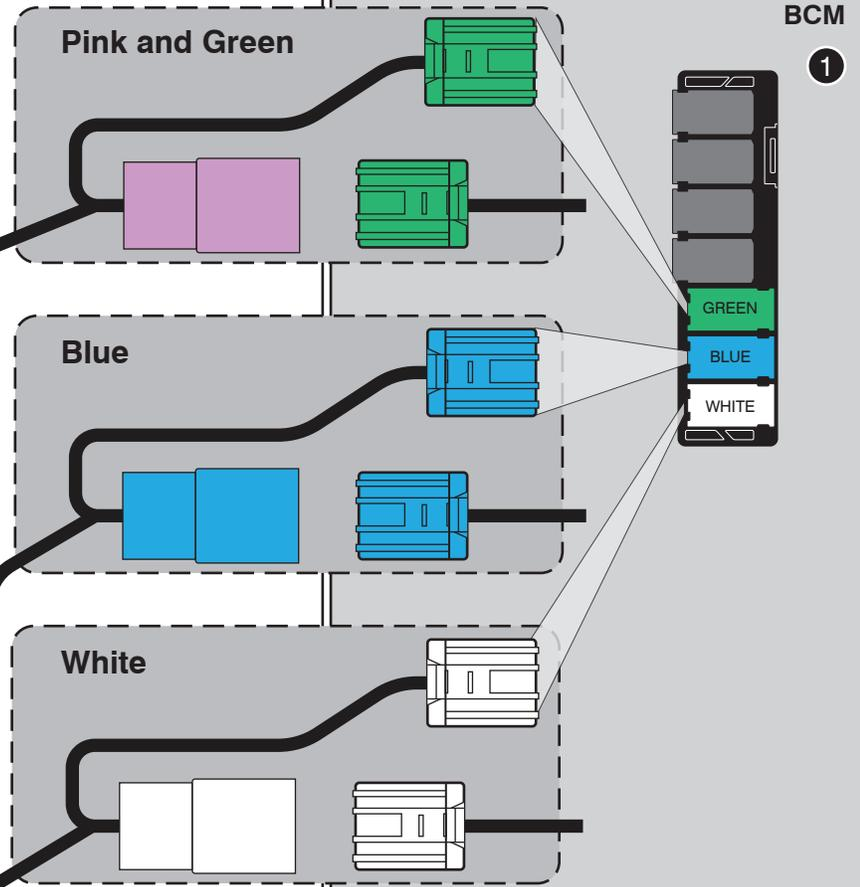
**E** Type 6 install requires an ACC pulse with disarm to properly control the OEM alarm system. **Set feature option 1-11 to option 3 (ACC pulse, same timing as disarm pulse)**
