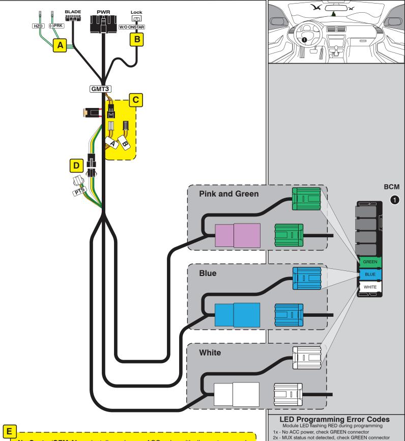
No Onstar/OEM Alarm install requires an ACC pulse with disarm to properly control the OEM alarm system. Set feature option 1-11 to option 3 (ACC pulse, same timing as disarm pulse)
