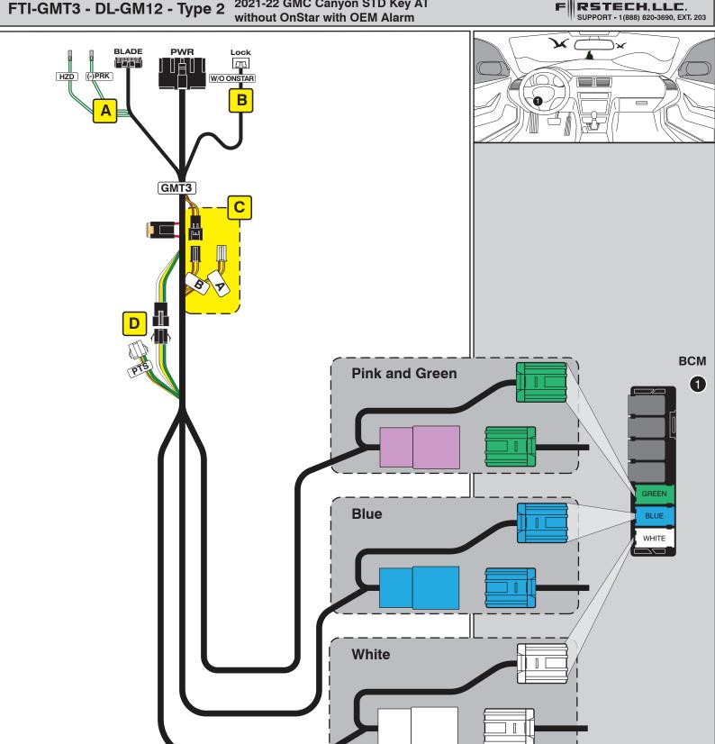
No Onstar/OEM Alarm install requires an ACC pulse with disarm to properly control the OEM alarm system. Set feature option 1-11 to option 3 (ACC pulse, same timing as disarm pulse)
