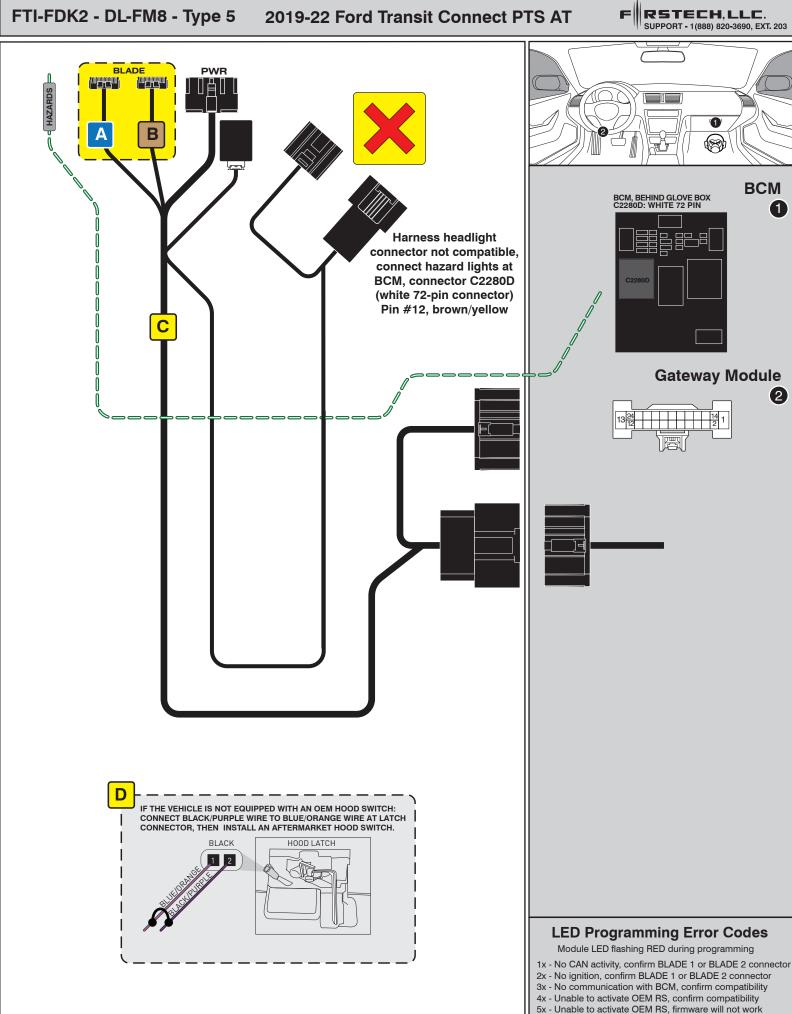
Fast Blink - CAN connection, reverse BLADE 1/2 connector
