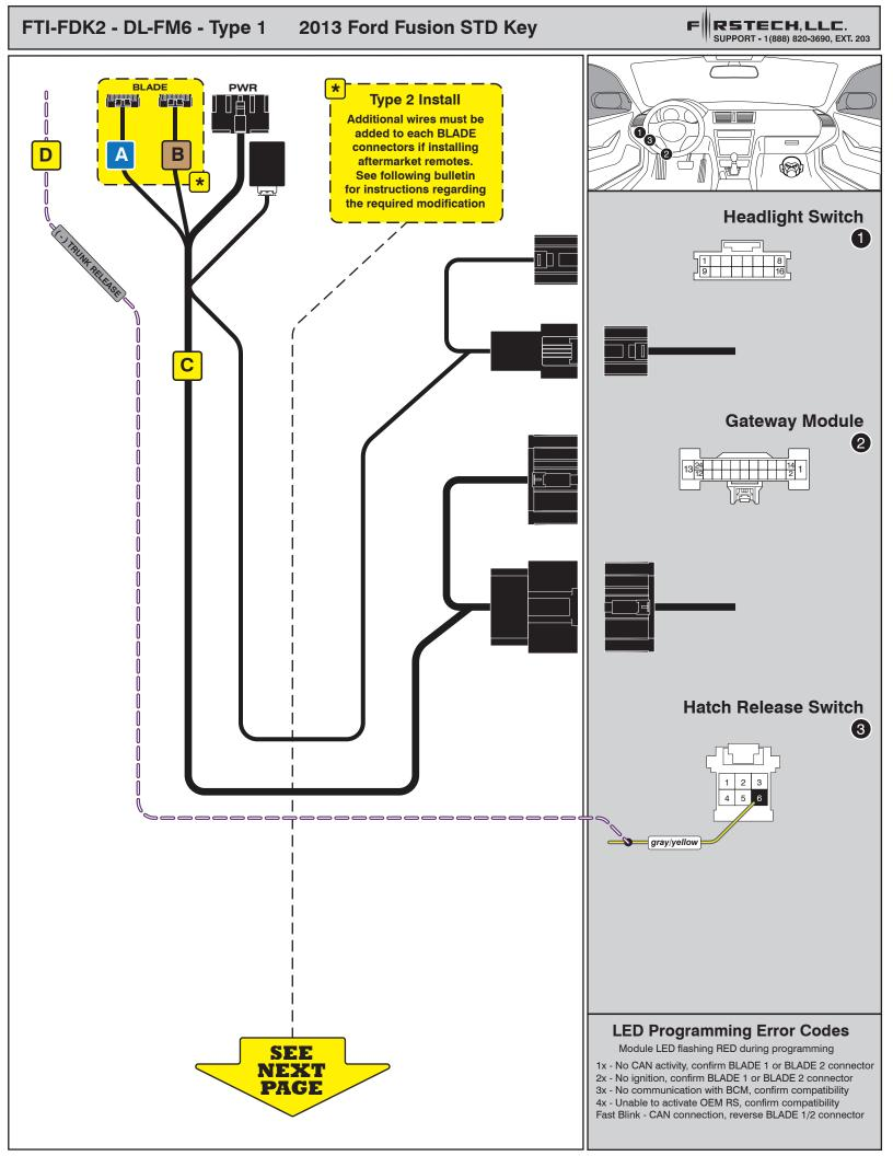
Overview: The initial production release of the FTI-FDK2 harness did not account for the use of aftermarket RF components and does not supply the connection that programs the module for aftermarket RF use. This issue affect the initial release and is currently being addressed in production, but for installations using aftermarket RF a field repair is provided below.
