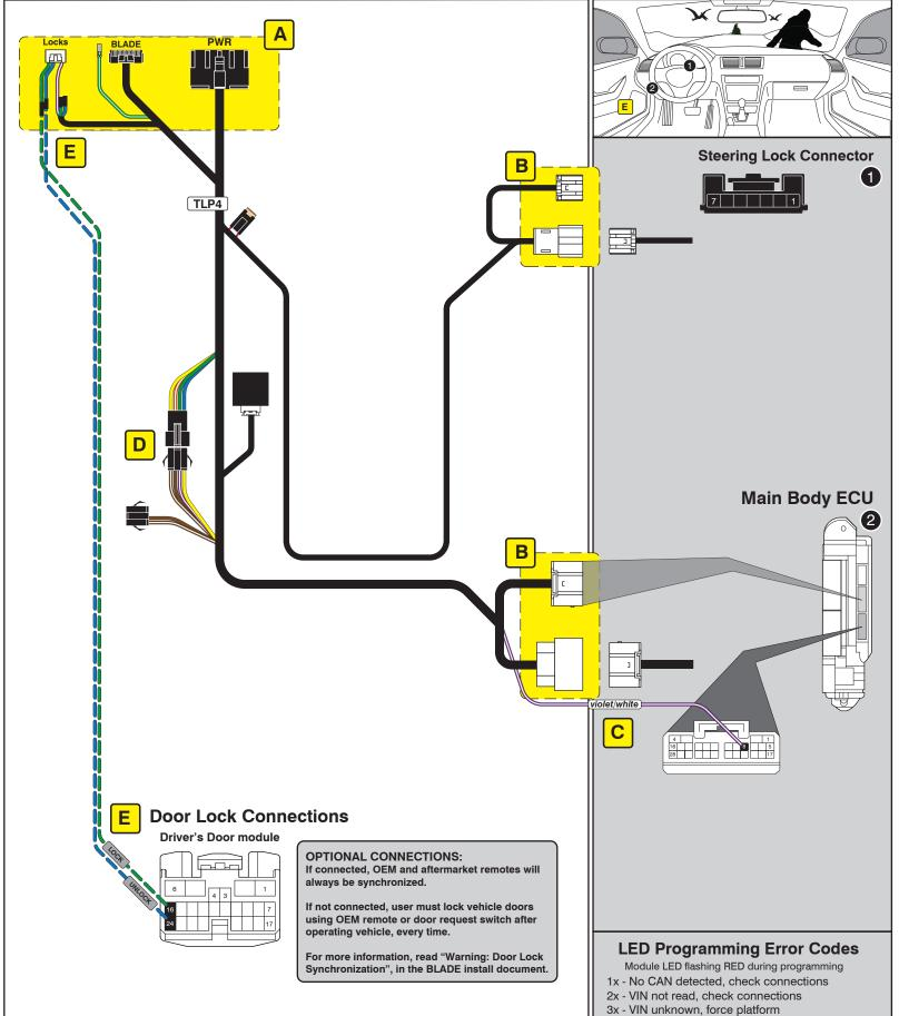
TAKEOVER NOT SUPPORTED: THE VEHICLE WILL SHUT DOWN UPON OPENING DRIVER'S DOOR
