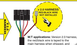
the red/black wire is taped to the main harness when shipped, and must be installed in the CN1 connector when installed.
