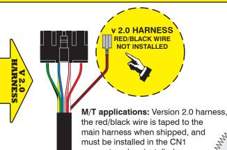
the red/black wire is taped to the main harness when shipped, and must be installed in the CN1 connector when installed.
